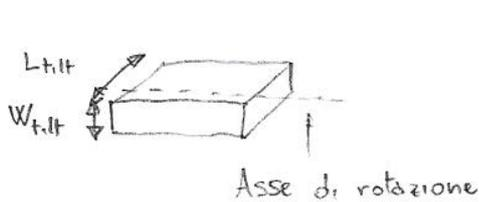
$$J_{\text{tilt}} = M_{\text{tilt}} \cdot \frac{L_{\text{tilt}}^2 + W_{\text{tilt}}^2}{12}$$
