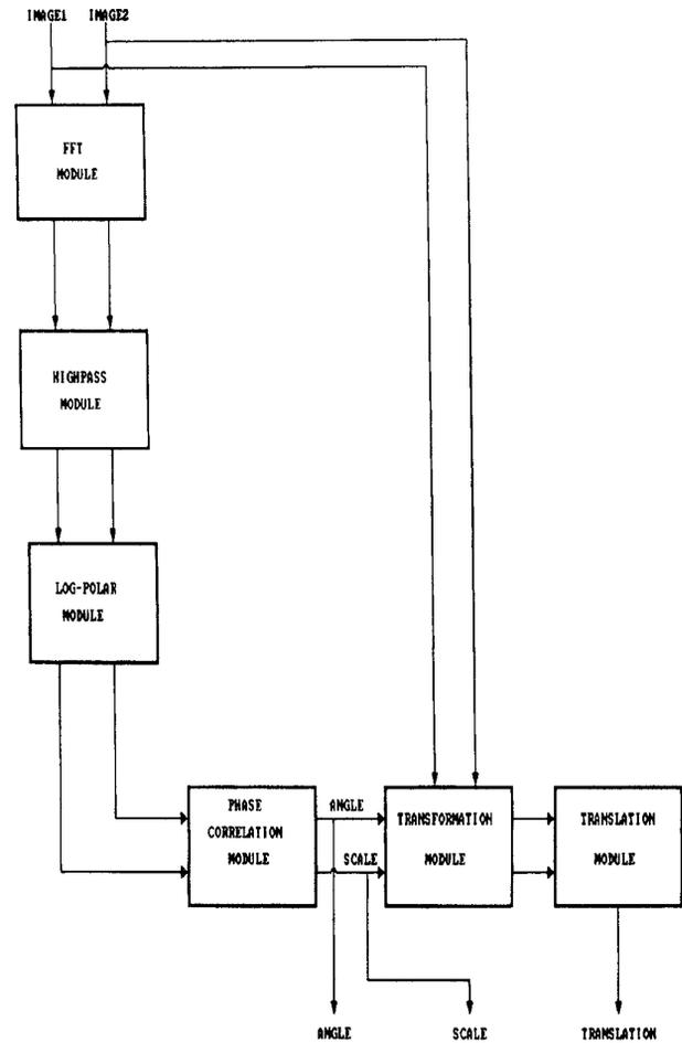
Fig. 1. Overview of the registration algorithm.
