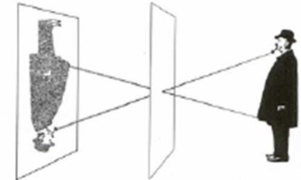
subject got through the tiny opening, producing a soft but acceptably clear photograph. Because of the small size of the pinhole, the exposure had to be 6 sec long.
