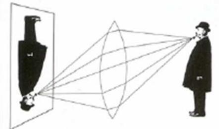
The lens opening was much bigger than the pinhole, letting in far more light, but it focused the rays from each point on the subject precisely so that they were sharp on the film.
